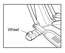
cal crosstrainer to the desired location and then lower it. Due to the size and weight of the elliptical crosstrainer, use extreme caution whilst moving it.
